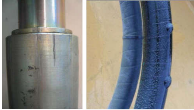
Fig. 258: Cracks on the clamping sleeve or blisters on the outer jacket
