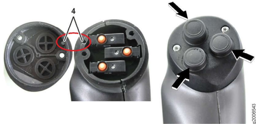
Fig. 189: Fitting the button cover
