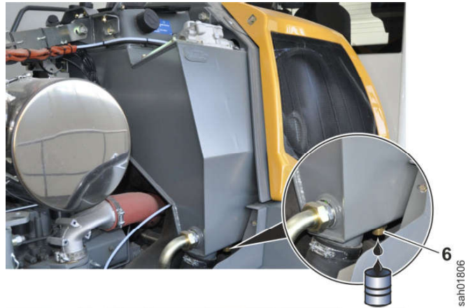
Fig. 163: Draining oil from the hydraulic tank
