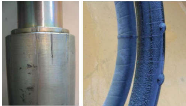
Fig. 167: Cracks on the clamping sleeve or blisters on the outer jacket
