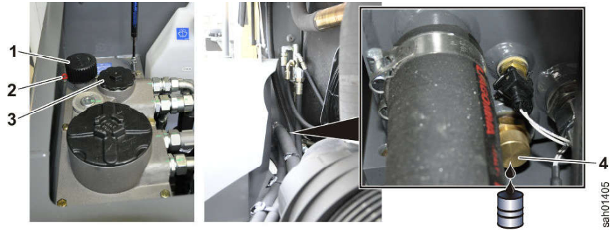
Fig. 96: Draining hydraulic oil
