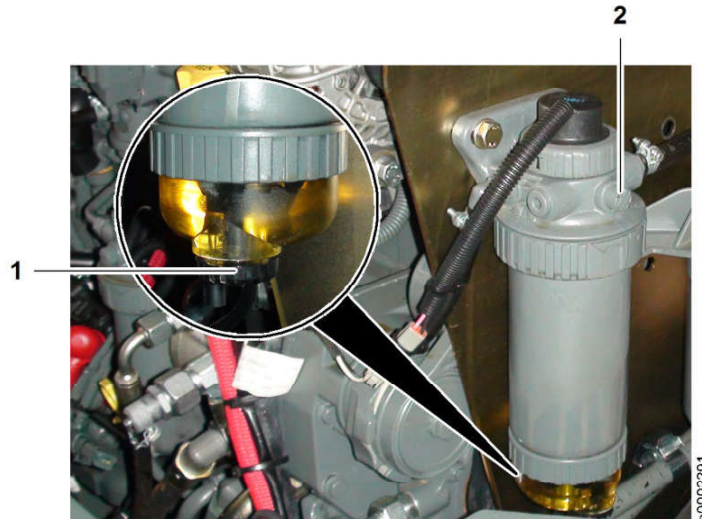
Fig. 52: Draining off condensate from the fuel pre-filter
