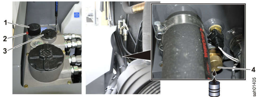
Fig. 89: Draining hydraulic oil
