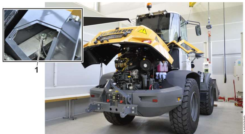
Fig. 145: Checking the antifreeze and corrosion inhibitor concentration
