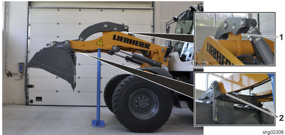
Fig. 198: Checking lift arm bucket stops
