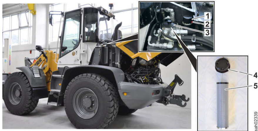
Fig. 160: Hydraulic tank: changing filter cartridge in return-suction filter
