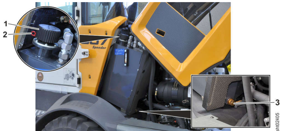
Fig. 202: Draining off condensate and sediment from the hydraulic tank
