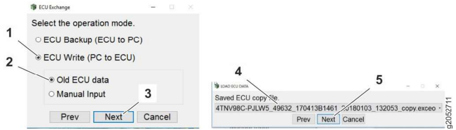
Fig. 233: Transferring setting data of old engine control unit
