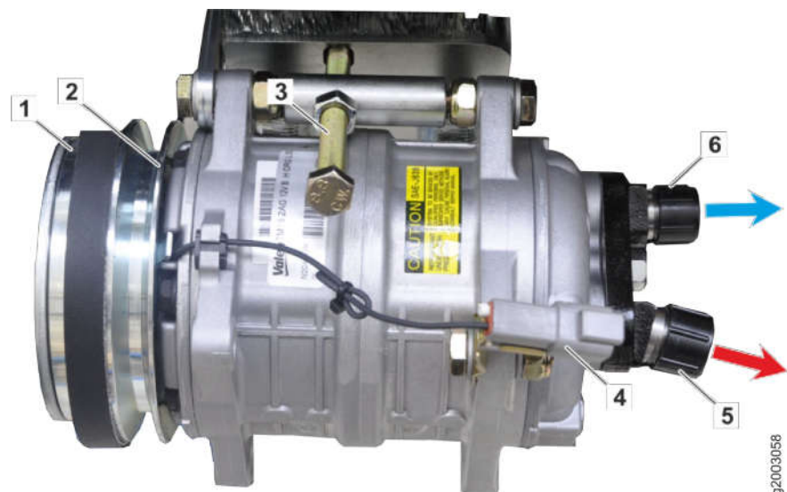
Fig. 499: Sectional view of air conditioning compressor
