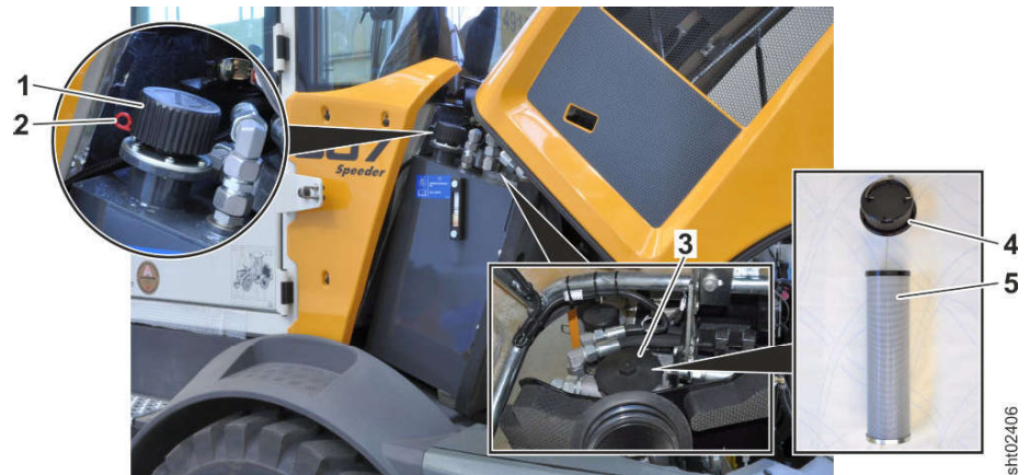
Fig. 137: Changing the hydraulic tank return suction filter cartridge
