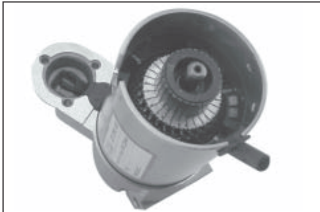
Figure 8-49. Installing Frame and Drain Tube.
