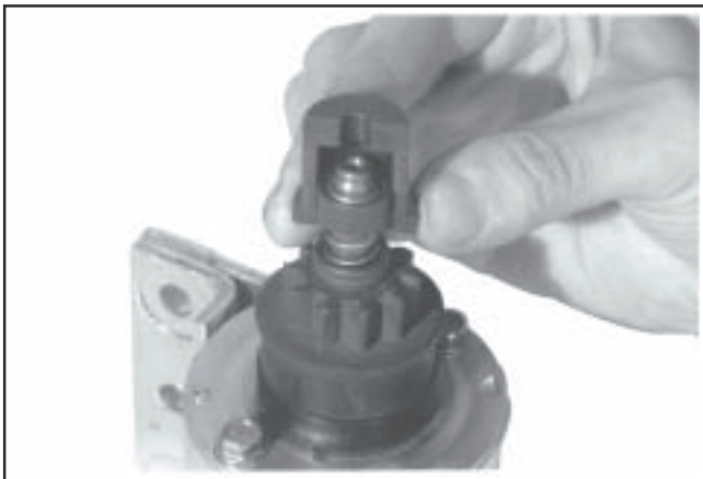
Figure 8-14. Assembling Larger Inner Half Around Spring Retainer.
