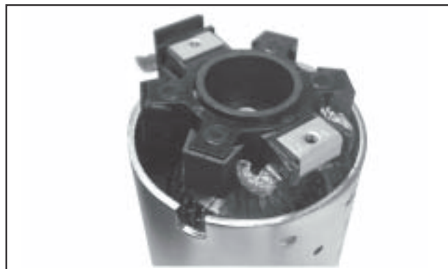
Figure 8-51. Installing Brush Holder Assembly with Supplied Tube.
