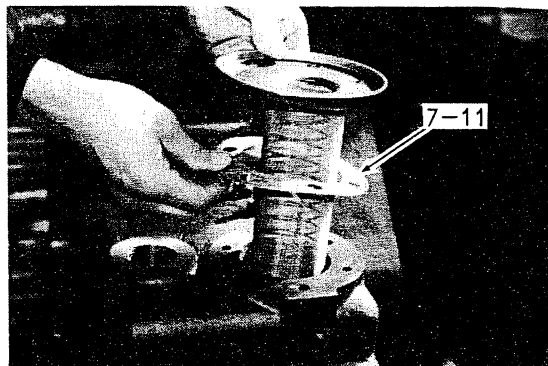
Fig. 5-4 Removal of Screen
