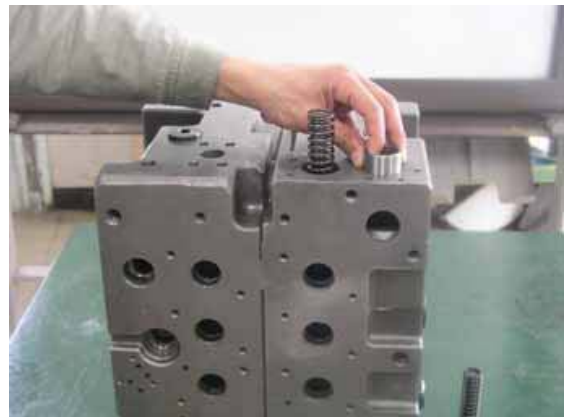
Removing boost check valve sub (517) and by-pass check valve poppet (518)
