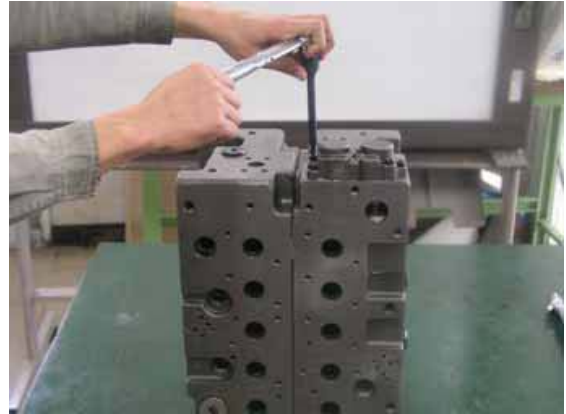
Removing back pressure check valve cover (207)
