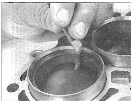
15.3 Measuring piston ring installed end gap
