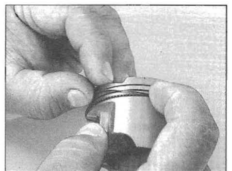
15.6b ... and fit the side rails each side of it. The oil ring must be installed by hand
