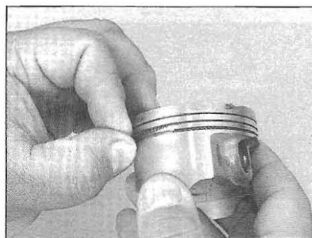
15.6a Install the oil ring expander in its groove, making sure the ends do not overlap ...
