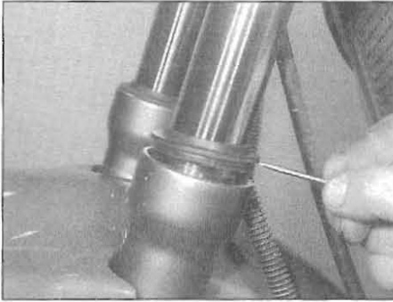
22.3 Checking for leakage of the fork seals
