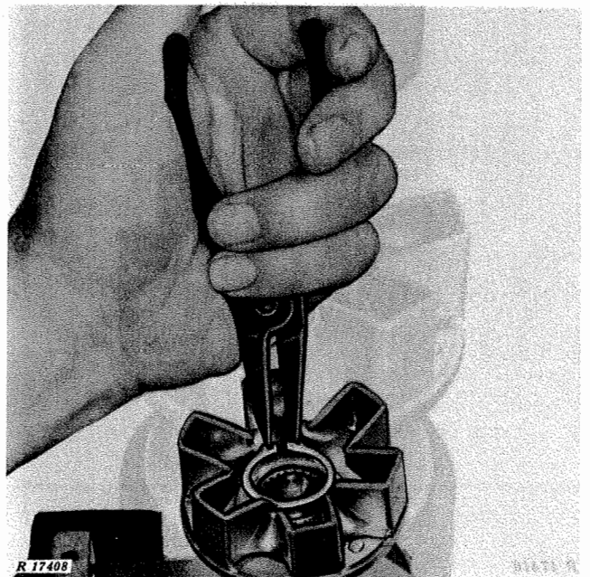
Fig. 11-15-31—Removing Snap Ring
