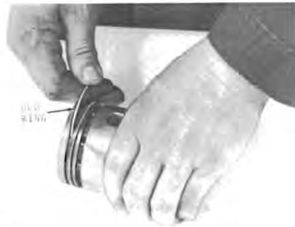
Fig. 12—Cleaning Ring Grooves
