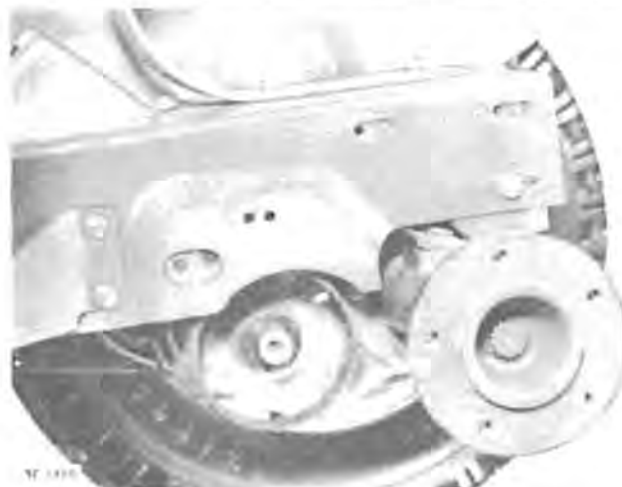
Fig. 30—Brake Bracket Used on Later 110 and All 112 Tractors
