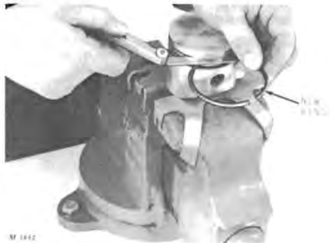
Fig. 13—Measuring Ring Clearance
