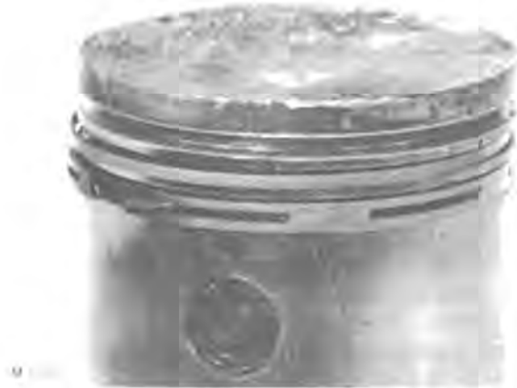
Fig. 13-Worn Oil Rings Which Cannot Provide Oil Control
