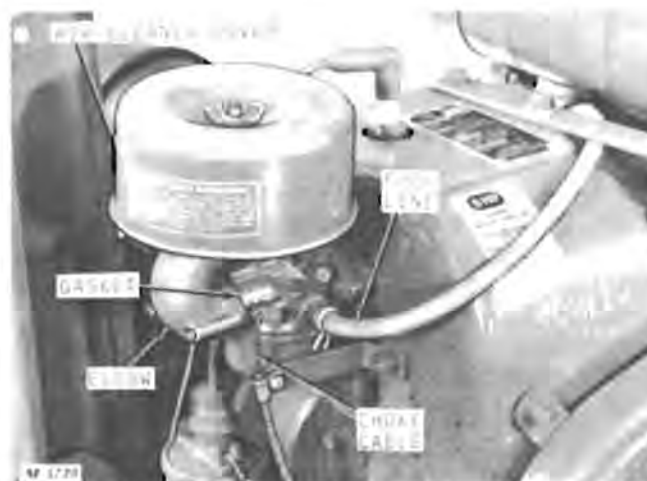
Fig. 8—Installing Carburetor Components
