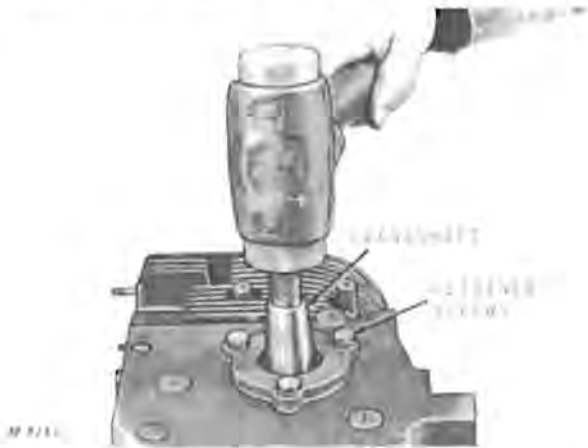
Fig. 37—Seating PTO Bearing
