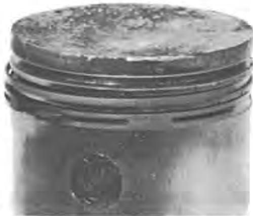
Fig. 11—Worn Oil Rings Which Cannot Provide Oil Control
