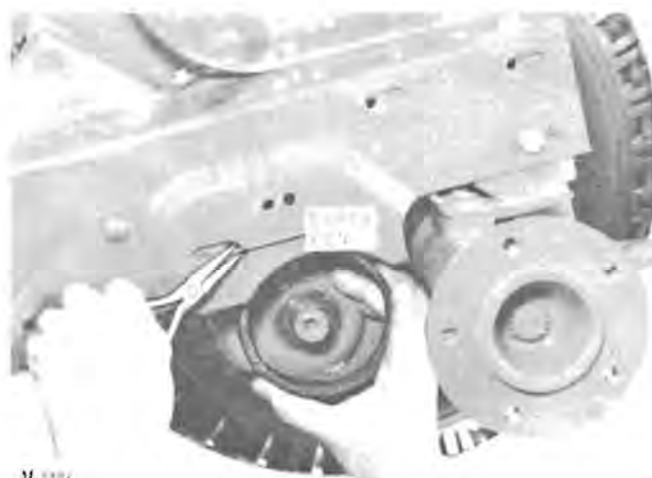
Fig. 31—Removing Brake Pin
