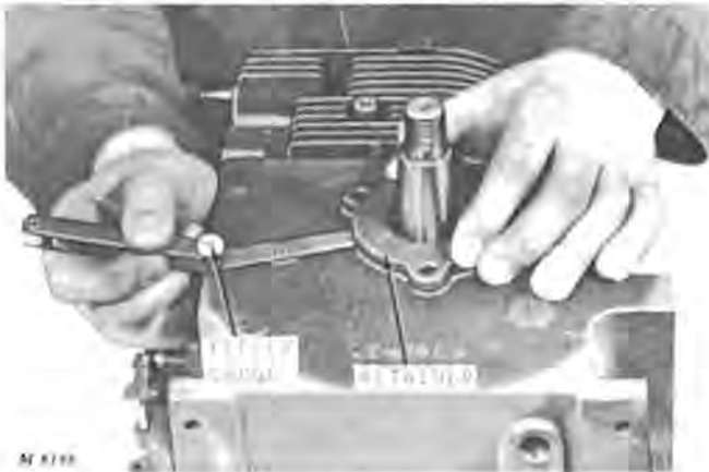
Fig. 38—Checking Gap Between Cylinder Block and Retainer
