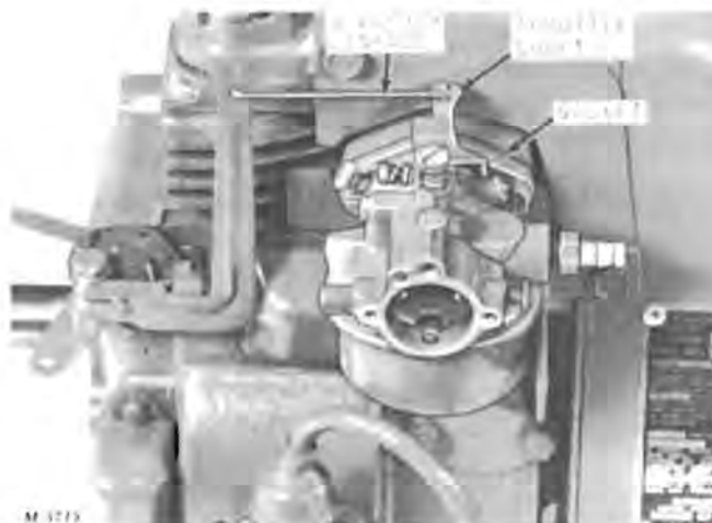
Fig. 7—Installing Carburetor Assembly to Cylinder Block
