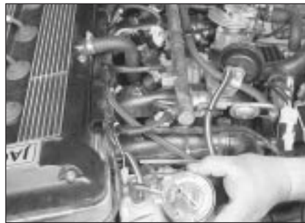
7.11b Check for vacuum from the TVV before and after the engine has reached normal operating temperature
