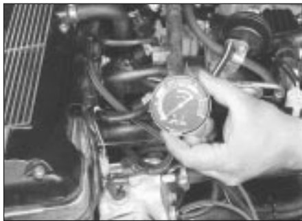
7.11a Check for vacuum to the thermal vacuum valve (TVV)
