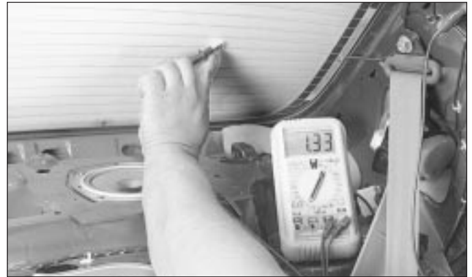
16.7 To find the break, place the voltmeter positive lead against the heated window positive terminal, place the voltmeter negative lead with the foil strip against the heating element at the positive terminal end and slide it toward the negative terminal end - the point at which the voltmeter reading changes abruptly is the point at which the element is broken
