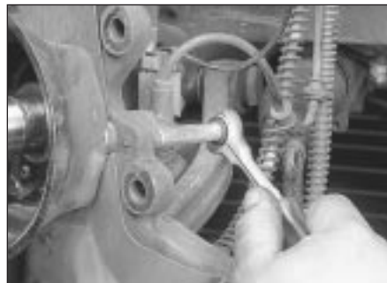
6.4 To detach the ABS sensor from the steering knuckle, remove this bolt
