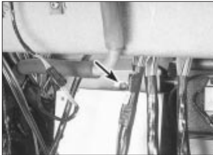
10.3b . . . then remove the upper ECU screw (arrowed) and pull down the ECU, then remove the ECU mounting plate
