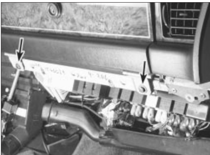
26.8 With the passenger side knee bolster removed, unscrew the glove box door hinge bolts
