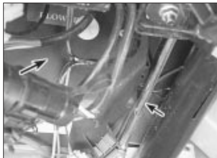
10.7 Remove this brace rod (small arrow) for clearance to remove the left blower motor housing (large arrow)
