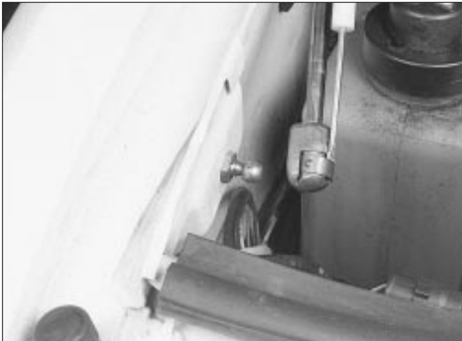
9.2a Use a small screwdriver to prise the clip out of its locking groove, then detach the end of the strut from the mounting stud
