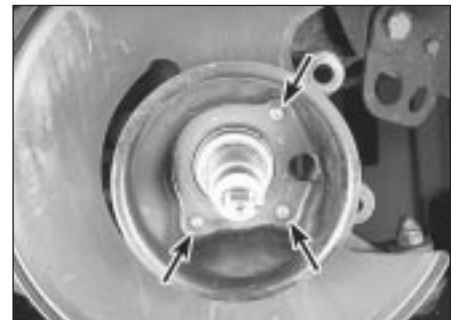
6.5 To detach the brake shield from the steering knuckle, remove these three screws (arrowed)
