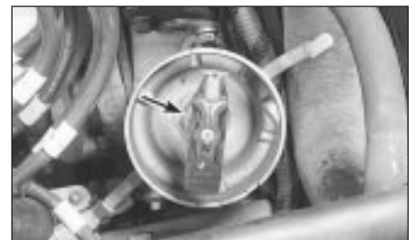
19.12a Pull off the rotor (arrowed) and inspect it thoroughly
