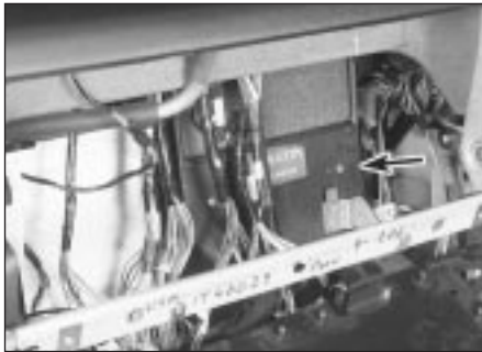
10.2a The right blower housing (arrowed) is located behind the glove box area of the dash
