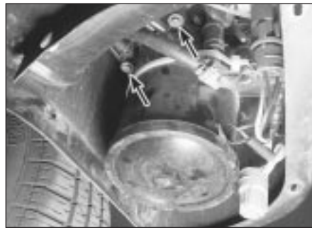
7.14 Remove the bolts (arrowed) and lower the charcoal canister from the wing
