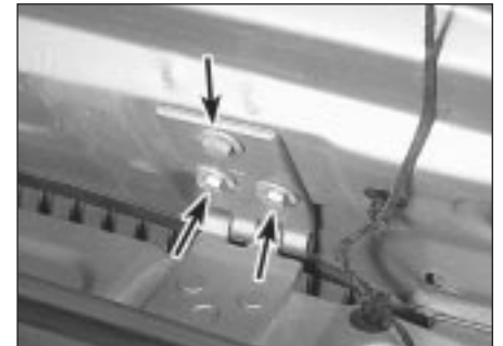
10.4 With the help of an assistant to hold the bonnet, remove the retaining bolts (arrowed) from each hinge plate, then lift off the bonnet
