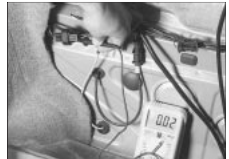
3.3b Check for battery voltage to the fuel pump on the harness connector near the fuel tank on models with in-tank fuel pumps
