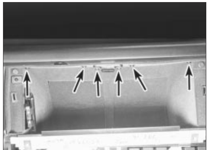
26.11 Remove the screws along the top edge (arrowed), pull the glove box out and remove the lamp assembly
