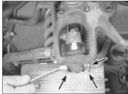
5.12 To detach the lower balljoint from the lower control arm, remove these four bolts (arrowed)
