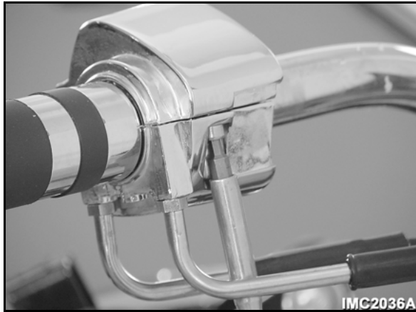
Figure 546 — Remove/install throttle/switch housing screws
