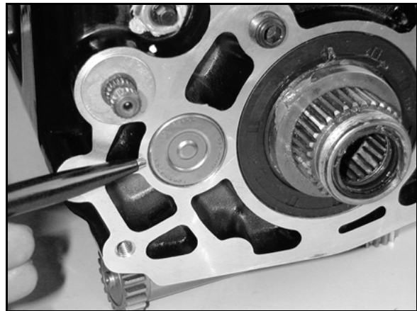
Figure 458 — Inspecting needle bearing at left of case
