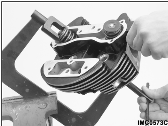
Figure 291 — Removing valves from cylinder head
