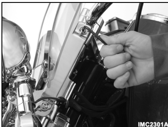
Figure 154 — Loosening mounting screws
