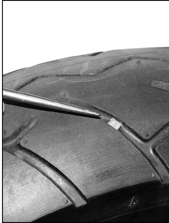
Figure 98— Wear indicator (painted for clarity)
