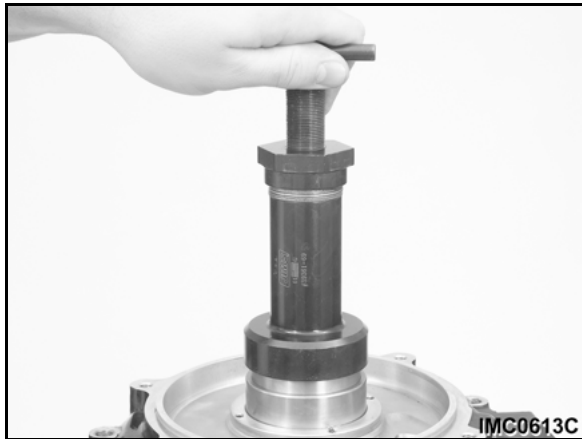
Figure 340— Seating seal in case
