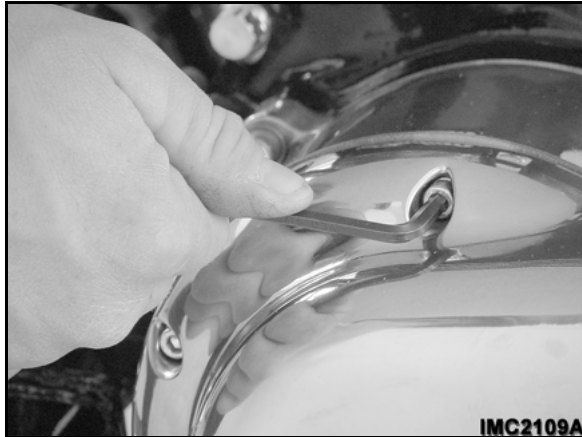
Figure 370— Tightening primary drive housing screws
