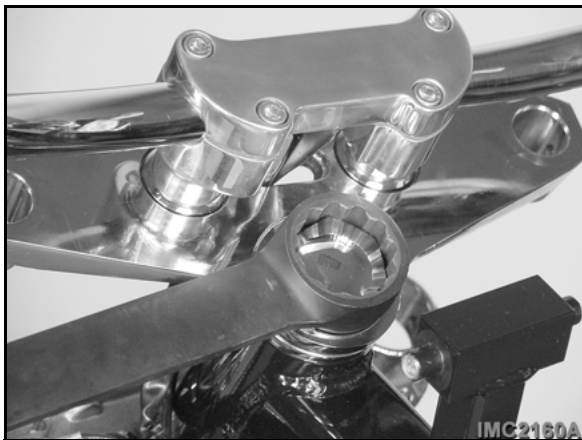
Figure 48— Crown nut removal
