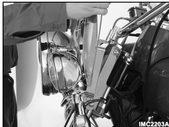
Figure 156 — Align bracket notches with mounting screws
