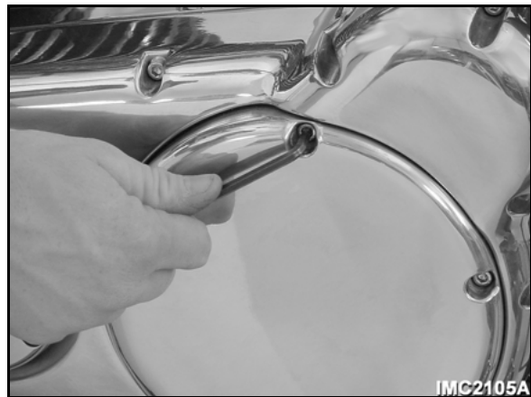
Figure 395 — Clutch cover removal
