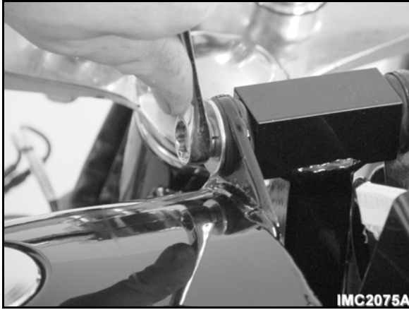
Figure 211 — Top-front mounting screw (left tank)
