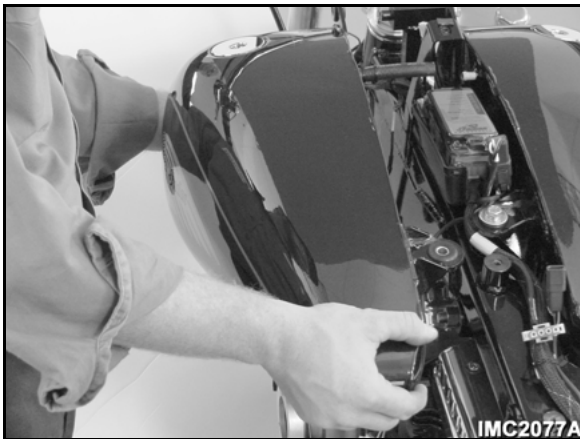
Figure 213 — Fuel tank removal (left shown)
