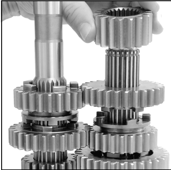
Figure 498 — Installing 5th gear onto countershaft
