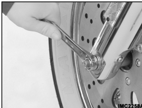
Figure 71 — Axle nut removal
