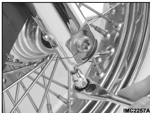
Figure 70 — Loosening pinch screw
