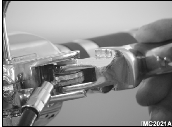
Figure 421 — Disconnecting clutch cable at handlebar control
