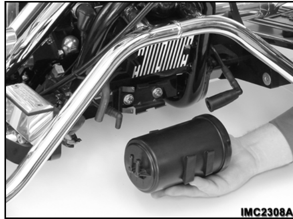
Figure 247 — Remove carbon canister
