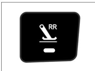
(12) Rear right outrigger switch
