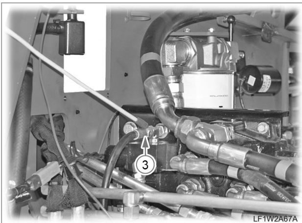
17. Install the return hose (3) between the main control valve and the oil tank.
