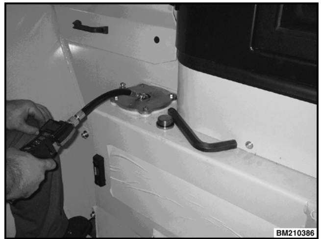
Figure 28. Hydraulic Oil Fill
