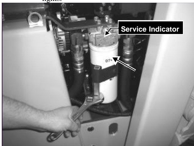
Fig. 8-28 Location of the rear hydraulic filter. Replace this filter when the service indicator above it shows, or reads, red.
