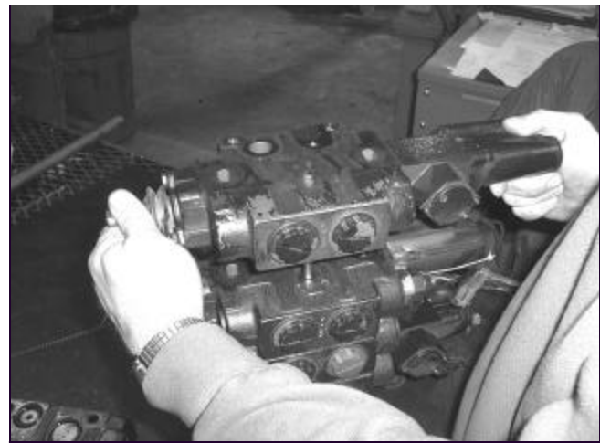
Fig. 8-86 One section of the control valve lifted off the valve stack bolts.
