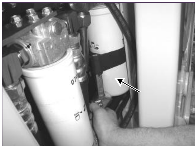
Fig. 8-27 Location of the forward hydraulic filter. Replace this filter when the restriction indicator light on the left instrument panel lights.
