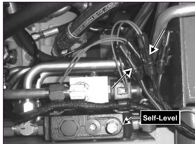
Fig. 8-57 Location of two electrical connectors on the tilt safety lock valve.
