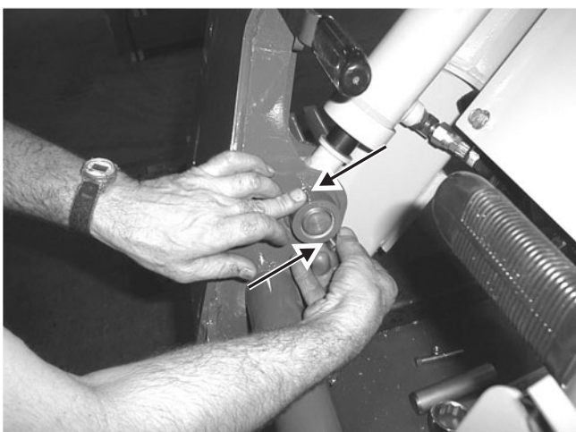
Fig. 8-32 Remove capscrew and locknut securing lower tilt cylinder pin to the All-Tach™.
