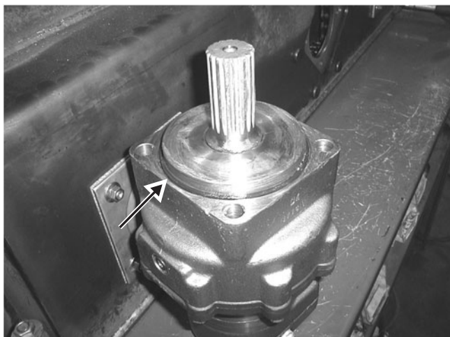
Fig. 7-23 Be sure o-ring seal is on drive motor prior to reinstallation into skid loader.
