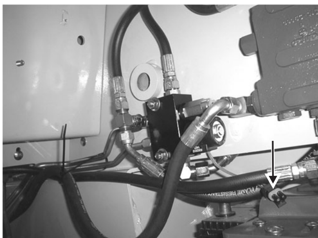
Fig. 10-41 One of three (1 of 3) hydraulic lock solenoids to electrically disconnect.
