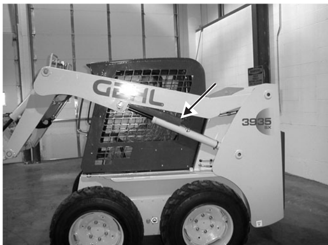
Fig. 2-3 Start the loader and raise the liftarm until the support device drops onto the lift cylinder rod, above the lift cylinder tube.
