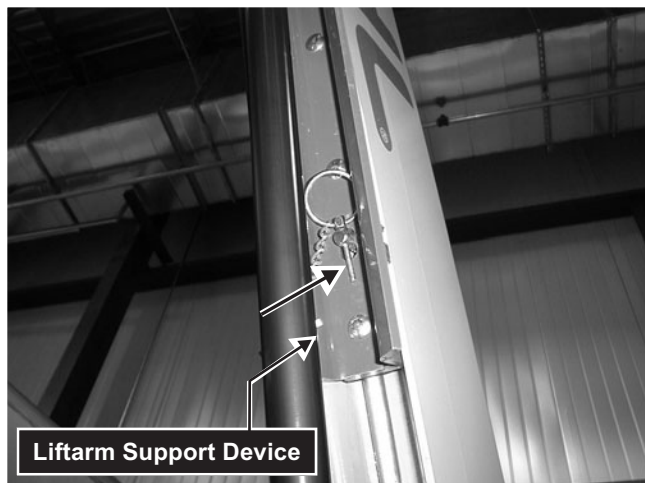
Fig. 2-1 The locking pin secures the liftarm support device underneath and inside the liftarm in the “storage” position.
