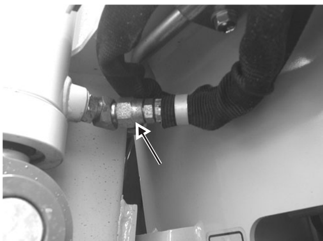
Fig. 8-11 Location of the lower hydraulic hose on the right tilt cylinder.
