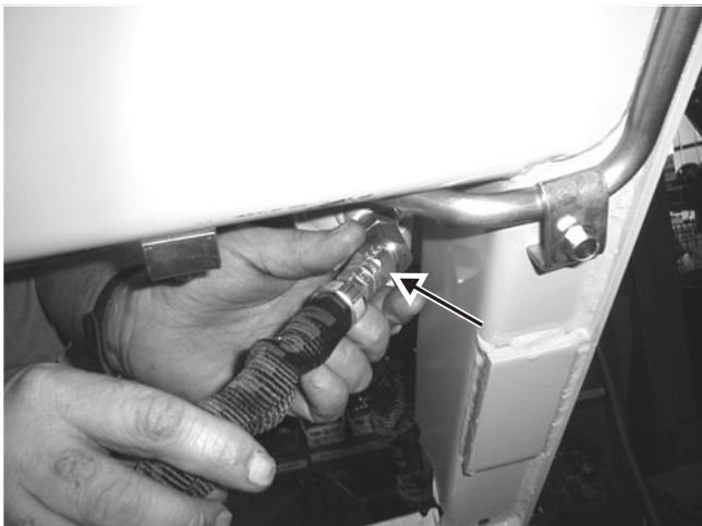
Fig. 8-31 Remove lower tilt cylinder hoses.
