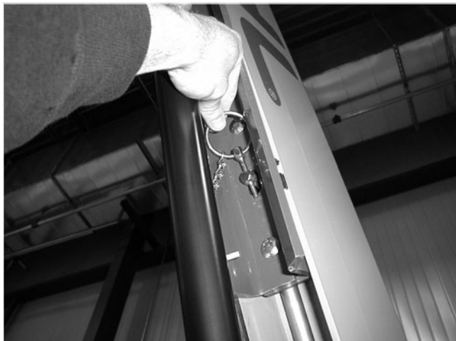
Fig. 2-2 Grab o-ring tether on locking pin and pull it out of the liftarm, allowing the support device to lie on the lift cylinder.
