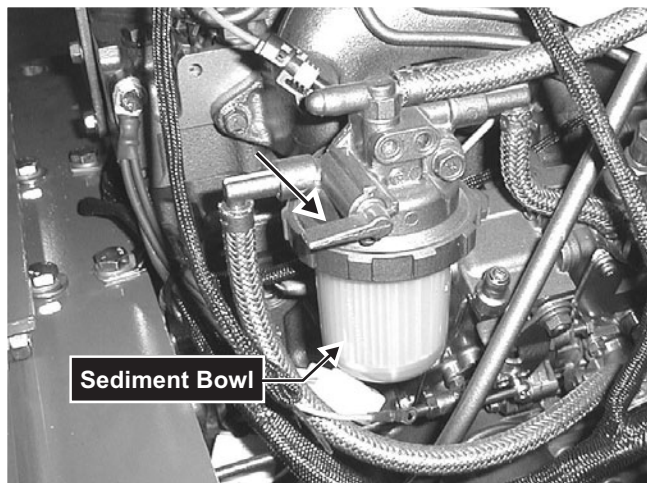
Fig. 10-12 Location of shut off valve on fuel filter.
