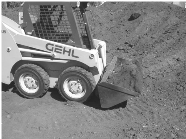
Fig. 8-9 For the tilt cylinder test, load a bucket with dirt, gravel or sand to begin the test.
