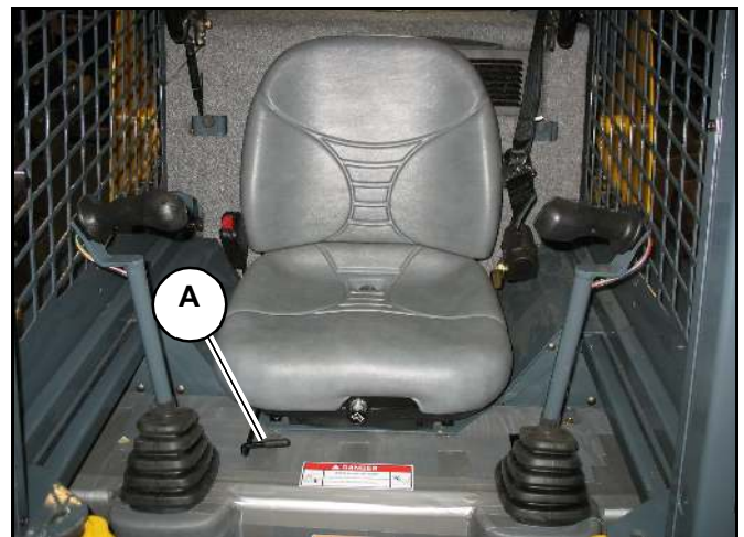
Fig. 2 – Operator's Seat Horizontal Adjustment
