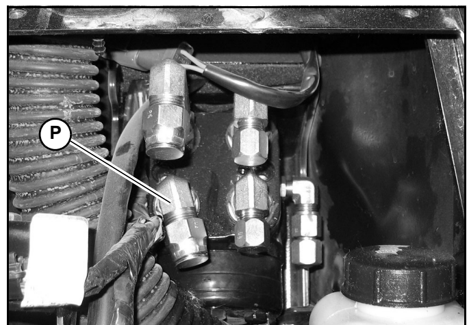
Fig. 165 – Steering Valve “P” Port (Hoses Shown Removed)
