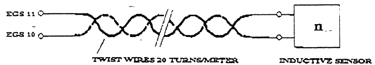
fig.5.4. Connection of an induction speed sensor with twisted cable
