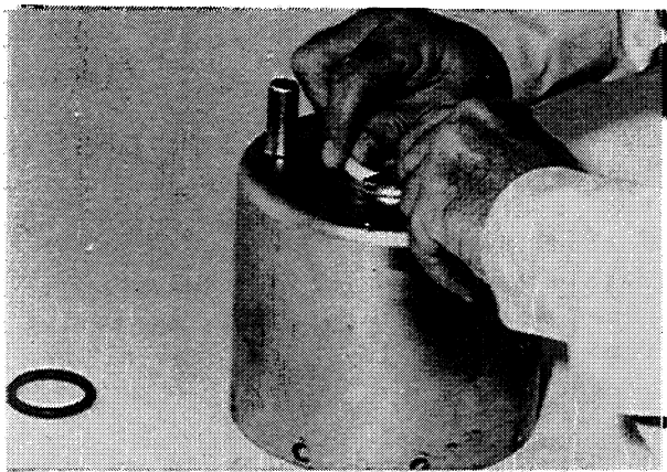
FIG. 54 SEALING CHAMBER T-84563
