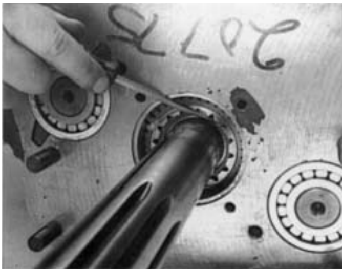
6. Remove the drive gear snap ring.
