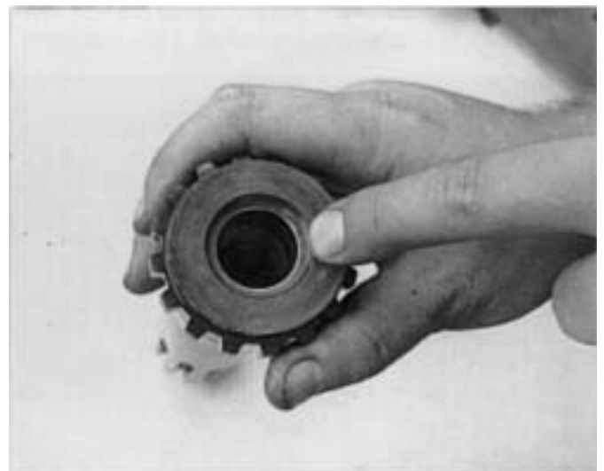
8. Check the bushing in the input shaft pocket, replace if worn.
