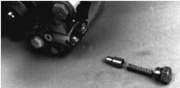
Fig. 50-34 - Heat Exchanger Bypass Valve (U)
