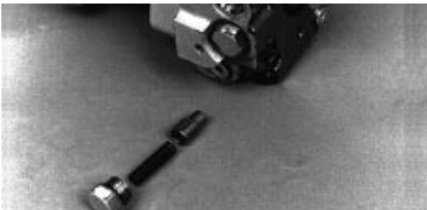
Fig. 50-36 - Filter Bypass Valve (U)
