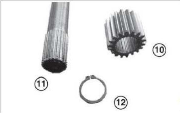
9. Remove snap ring (12) and then, remove sun gear (10) from the shaft (11).
