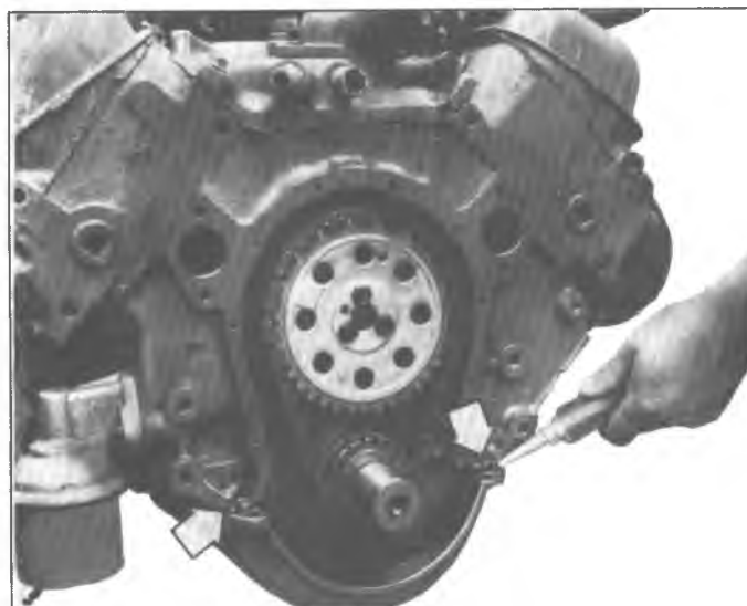
Fig. 18V—Applying Front Cover Sealer
