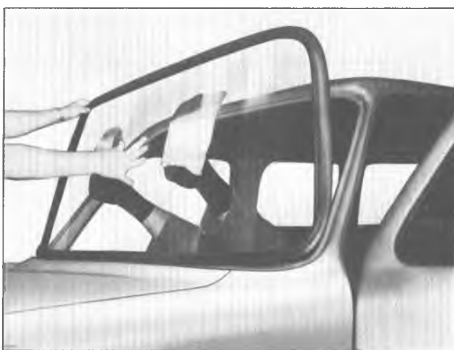
Fig. 16—Removing Windshield from Opening
