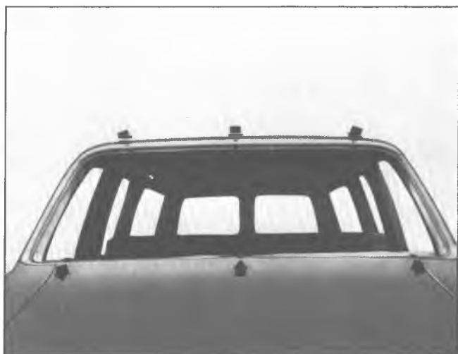
Fig. 17—Checking Windshield Opening
