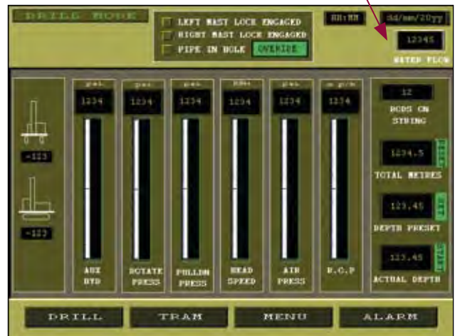
Water Injection Flow (Drill Mode Screen)
