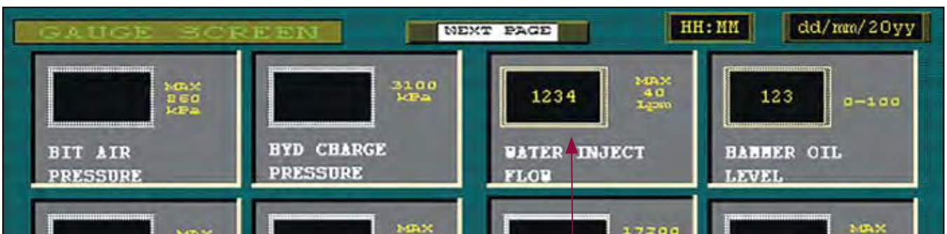
Water Injection Flow (Gauge Screen)
