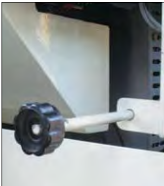
Water Controller – controls hydraulic flow to water injection pump
