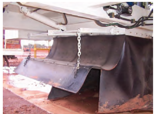
Dust Curtain Raised
