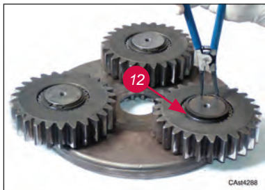
Disassemble snap ring (12).
