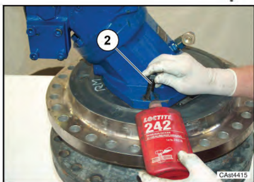
Apply Loctite® 242 on screws (2).
