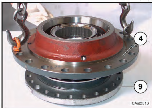
Assemble hub assembly (4) on beam assembly (9).
