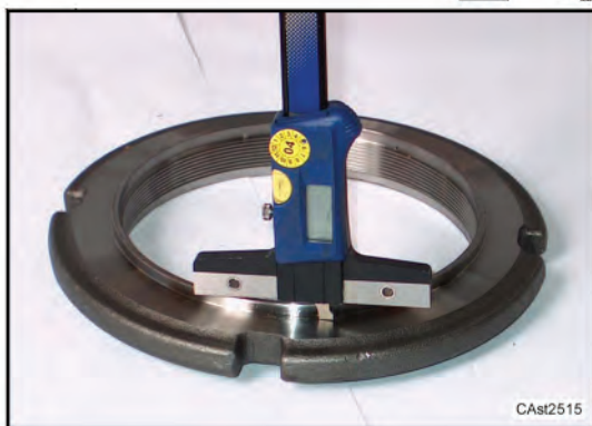
Measure the value (Y) on a new ring nut.
