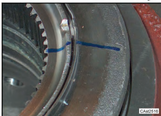
Screw completely the new ring nut without shims and draw a line of reference between the wheel hub carrier and the ring nut.
