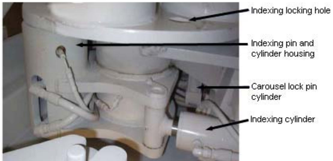
Fig. 6-34 Carousel Indexing Assembly
