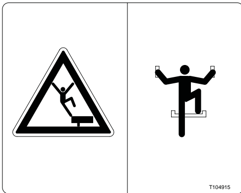
Fall Hazard (T104915)
