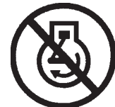
Engine STOP (also By-Pass)
