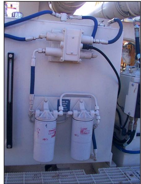
Fig 4-7: Engine Oil Reserve Assembly
