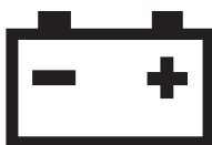
Voltage (Battery Charging)
