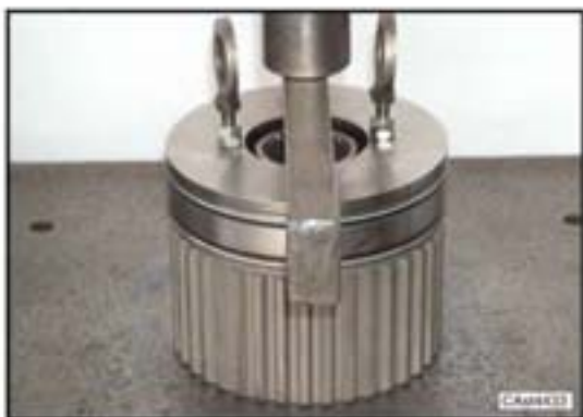
Assemble nr.2 eyebolts M6 to fasten the disc.
