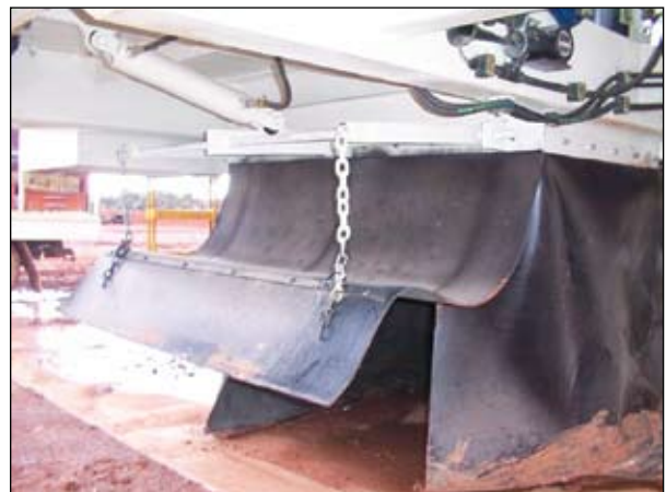
Dust Curtain Raised
