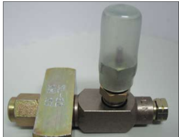
SI-32 Injector With Protective Cover SL-32 output with indicator cap hand-tightened is .016cc (.001cu. in.). Maximum output is achieved with five turns at .0014cu. in. / turn.
