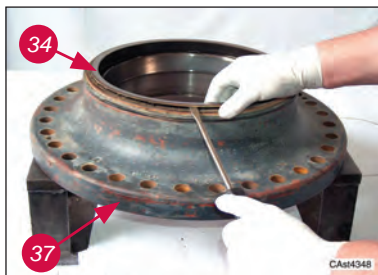
Assemble half gasket (34) from hub (37).
