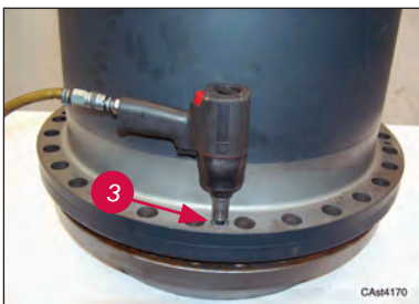
Unscrew and remove screws (3).
