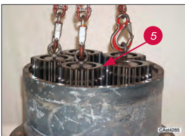
Remove planetary gears carrier assembly (5).
