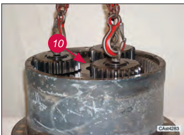
Remove planetary gears carrier assembly (10).
