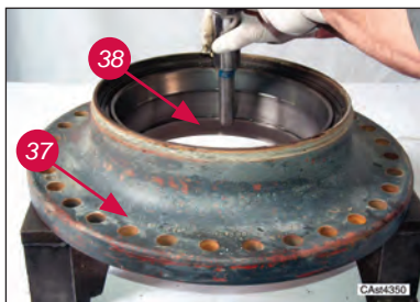
Remove bearing cup (38) from hub (37).
