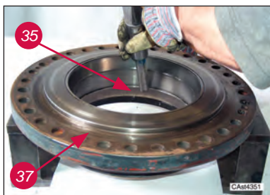
Remove bearing cup (35) from hub (37).
