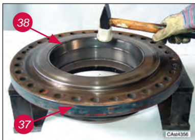
Assemble bearing cup (38) on hub (37).
