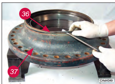
Assemble outer gasket (34) from hub (37).
