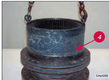
Remove hollow wheel (4).
