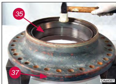
Assemble bearing cup (35) on hub (37).
