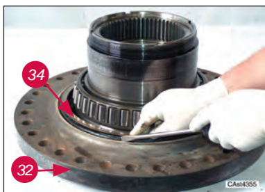
Assemble half gasket (34) on beam (32).
