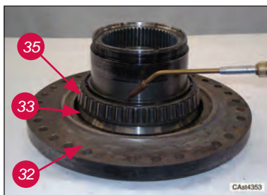
Remove bearing (35). Remove spacer (33) from beam (32).
