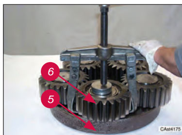
By means of an extractor remove planetary gears (6) from side gear carrier (5).
