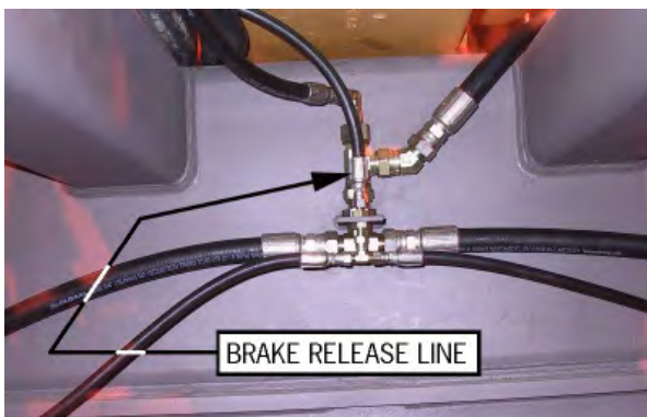
Fig. 7-8a Brake Release Line at Tee Fitting. Located just above axle pivot beam.
