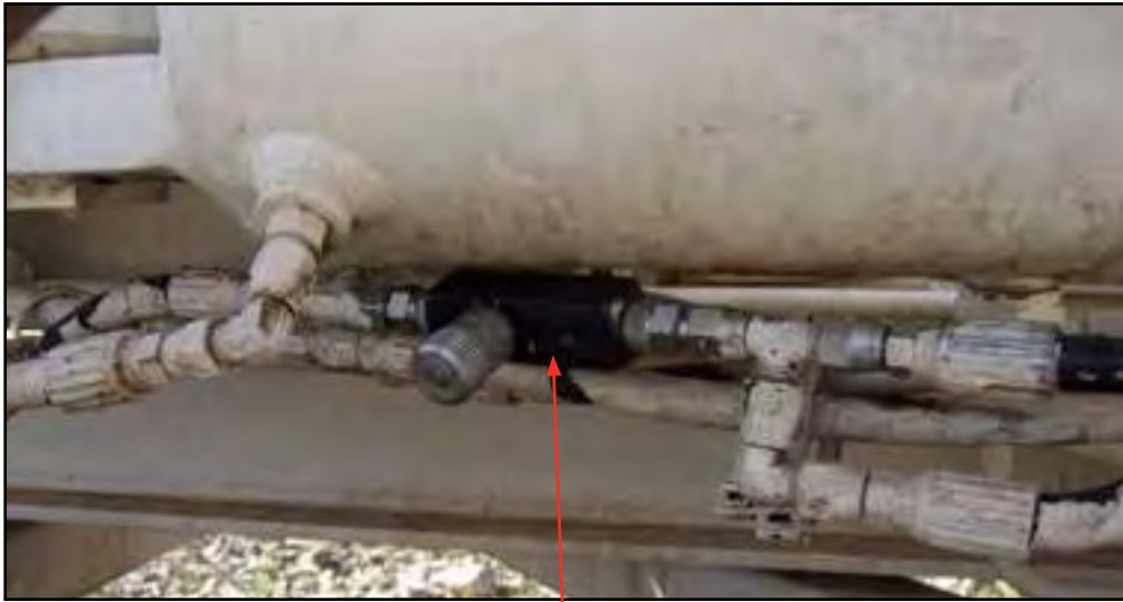
Needle Valve with locking screw
