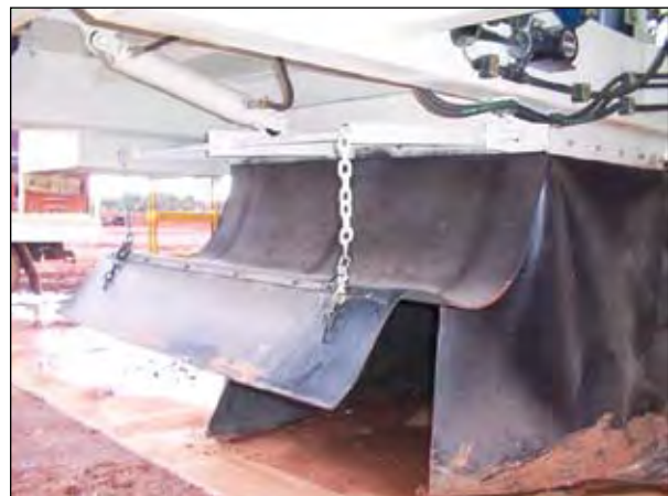
Dust Curtain Raised
