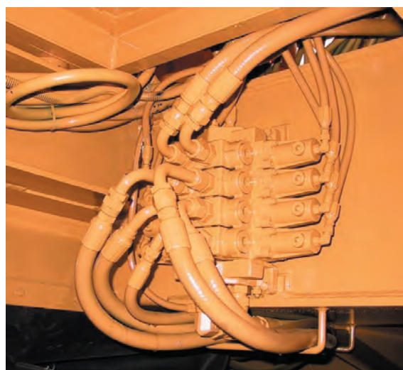
Fig. 7-14 Mast Elevate & Jack Control Valve 410091 (mounted under operator's cab)
