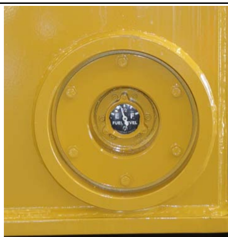
FUEL TANK INSPECTION COVER AND LEVEL GAUGE, DRAIN PLUG UNDERNEATH
