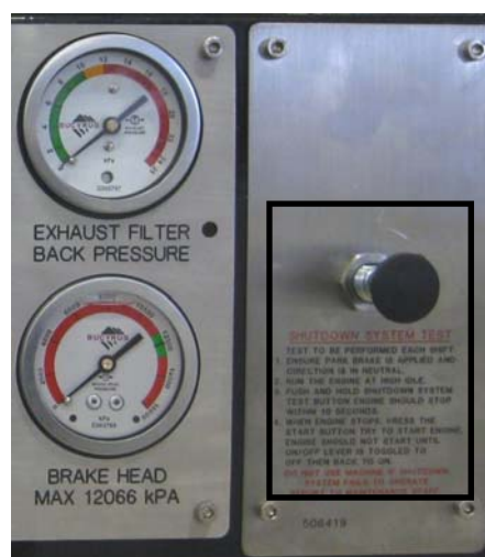
SHUTDOWN SYSTEM TEST VALVE
