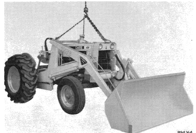
Figure 69 - Chain Hoist Attachment
