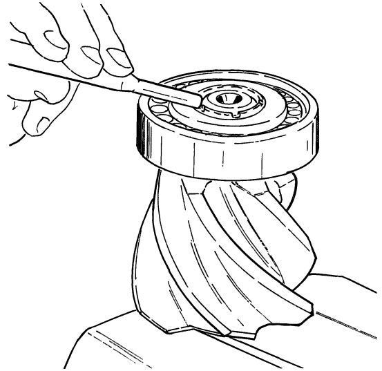
Figure 10. Bending the Crimping to the Inner Side
