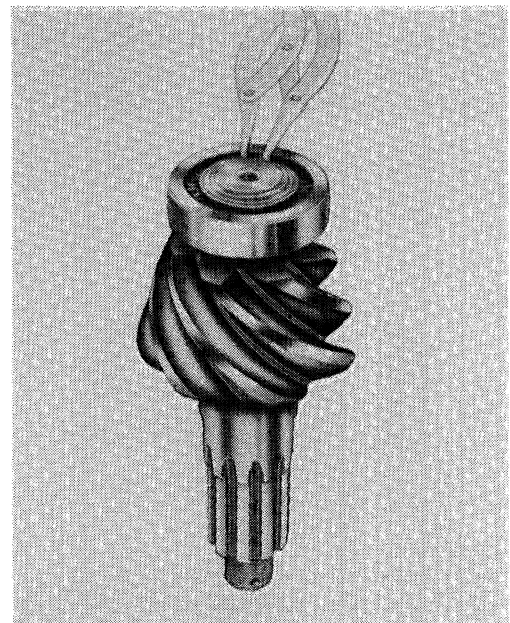
Figure 10. Removing Bearing Snap Ring
