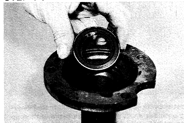
Press a new oil seal in clutch throwout spindle until it bottoms.
