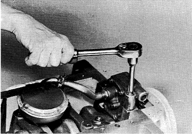
Remove oil pump mounting bolts.
