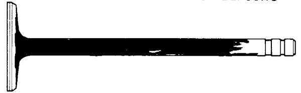
HEAVY CARBON AND VARNISH DEPOSITS
